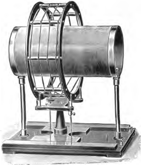
High frequency transformer.
